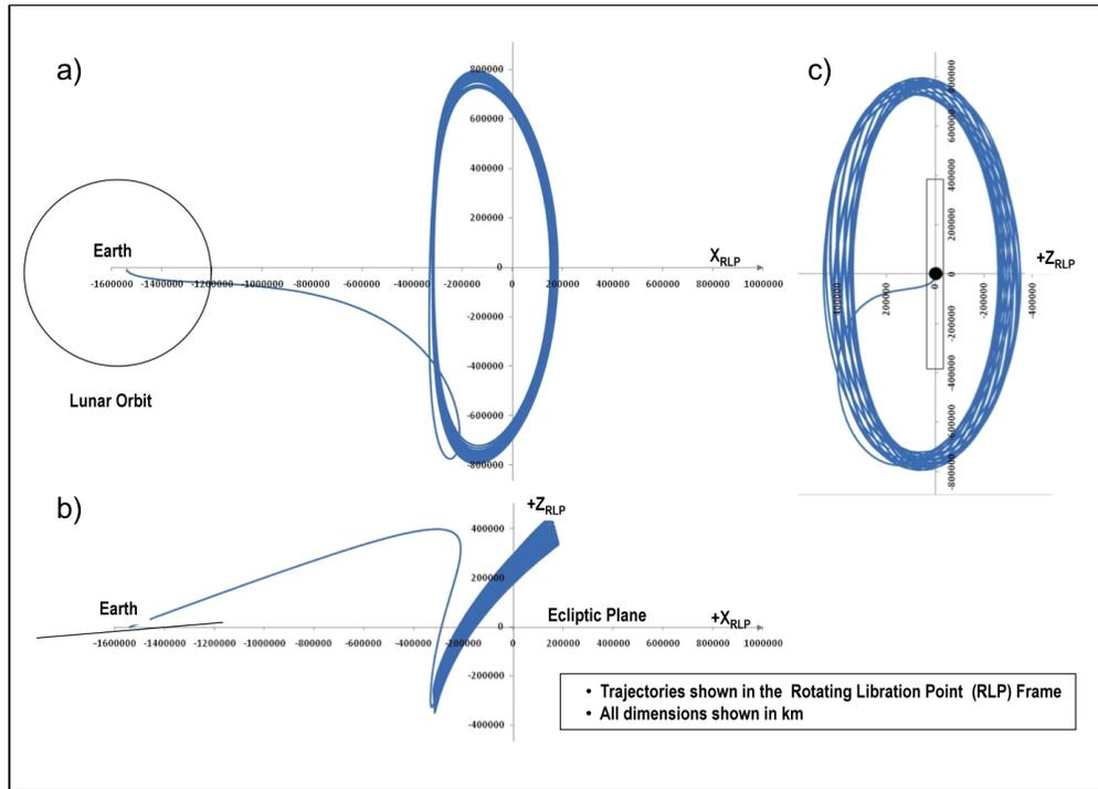
*A representative example of a valid JWST trajectory and orbit. Panel a is the view of the orbit projected onto the ecliptic plane; panel b is the view in the ecliptic plane, and panel c is the view along the Earth-Sun line.*
