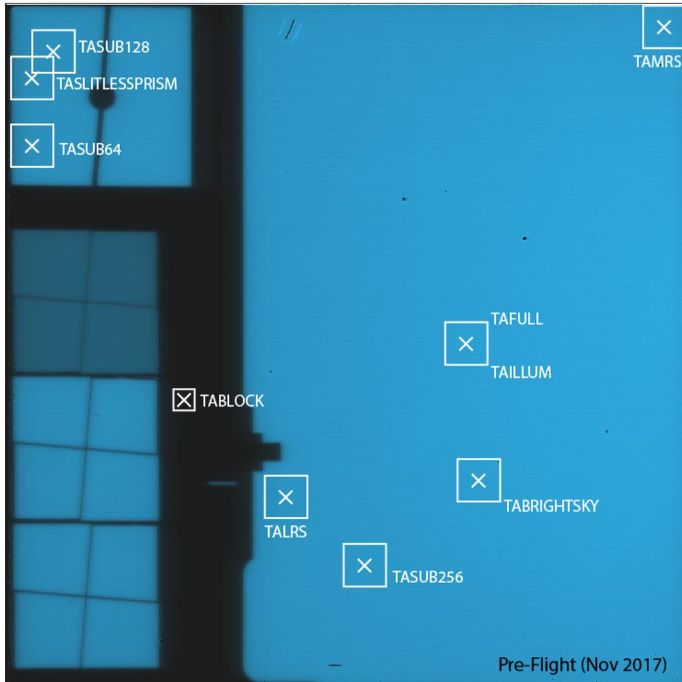
*The box labeled "TASLITLESSPRISM" in the imager region is where the LRS slitless target acquisition  $64 \times 64$  pixel region of interest (ROI) is located. The reference point is taken to be the midpoint of this ROI.*
