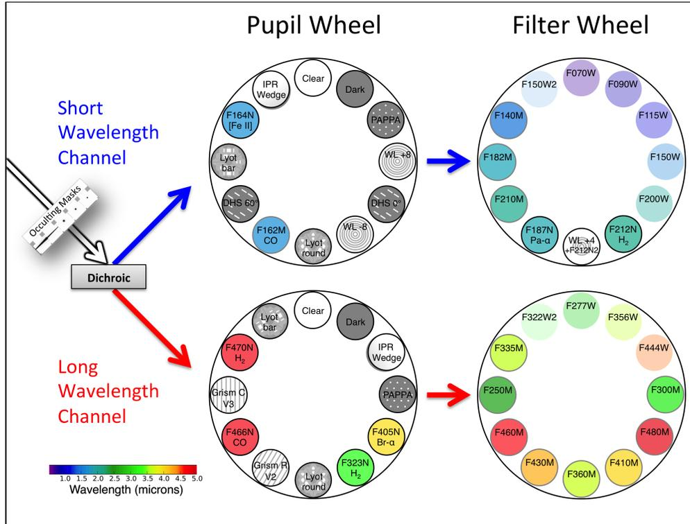
Each NIRCams module contains the optical elements depicted above, including pupil and filter wheels that hold a total of 48 optical elements. Filters are color-coded by wavelength. Wider filters are shown in the figure as more transparent than narrower filters.
