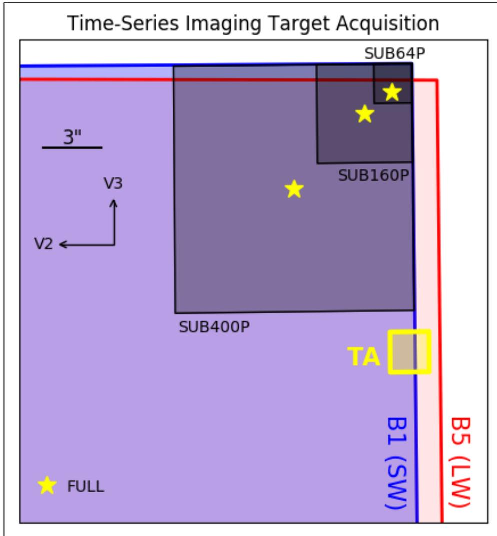
*Target acquisition is performed with a  $32 \times 32$  pixel subarray (yellow square) on the long wavelength detector B5, near the point source subarrays. The target acquisition pointing is centered on the TA subarray, followed by a telescope slew to one of the yellow stars at the center of the SW subarray for the science exposures. For simplicity, only the SW subarrays are shown here. For information on the location of the LW subarrays, see the [NIRCam Detector Subarrays](#) article.*
