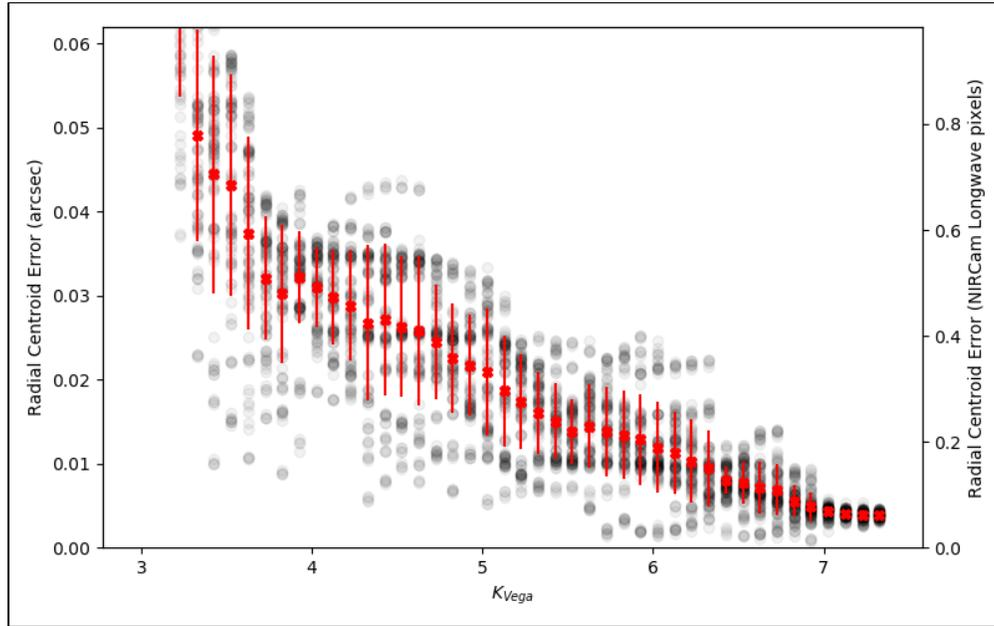
*Accuracy of the target location algorithm results for NIRCam time-series and grism time-series observations versus the K band Vega magnitude of a G2V source. The accuracy is calculated for a grid of subpixel locations and Poisson noise realizations. Individual results are shown as gray points. Red points and error bars show the mean and standard deviation over all pixel phases and noise realizations at each magnitude.*
