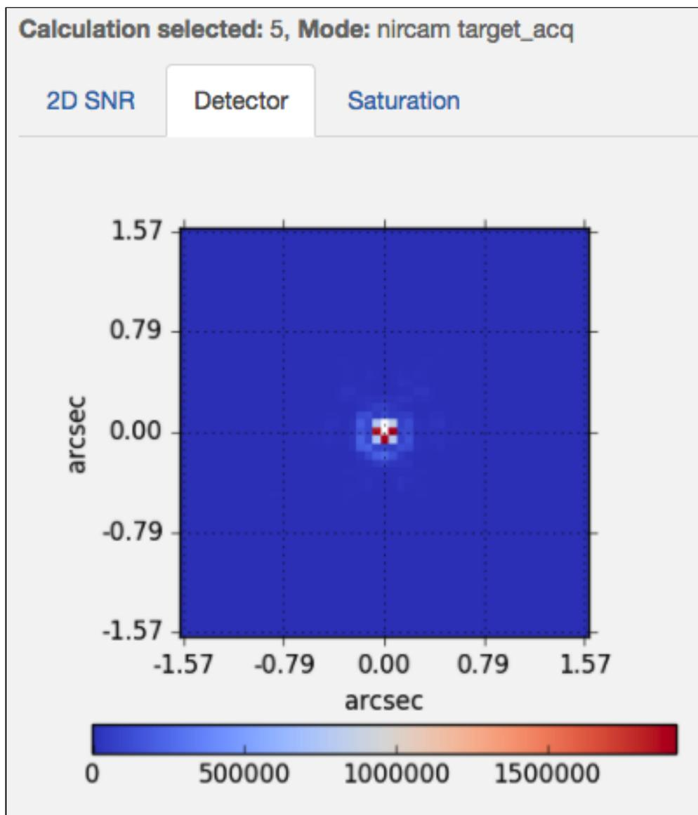
*Three pixels are saturated in the shortest (RAPID readout,  $N_{Groups} = 3$ ) target acquisition image of GJ 436. Using a narrow filter would prevent this, but that is not yet implemented for Cycle 1.*
