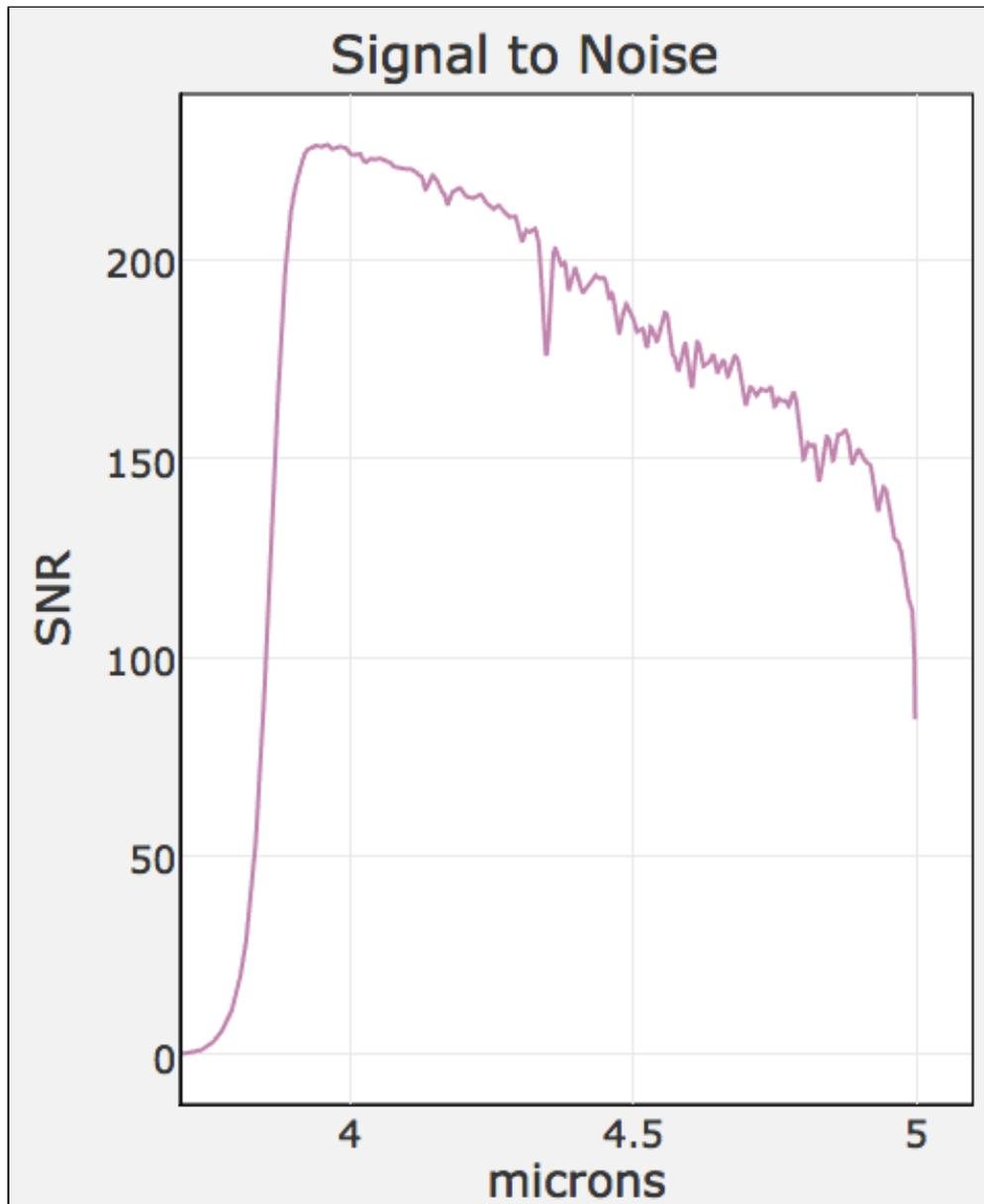
*The SNR plots for F322W2 + grism and F444W + grism observations generated by JWST ETC 1.1.1. F322W2 + grism observations (upper panel) will have SNR ~ 180 per spectral pixel in each 2.04 s integration, while the F444W + grism observations (lower panel) have SNR = 195 per spectral pixel in each 3.75 s integration.*
