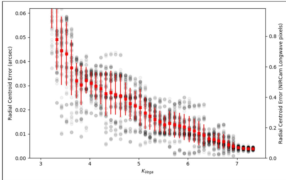
*Accuracy of the target location algorithm results for NIRCcam time-series and grism time-series observations versus the K band Vega magnitude of a G2V source. The accuracy is calculated for a grid of subpixel locations and Poisson noise realizations. Individual results are shown as gray points. Red points and error bars show the mean and standard deviation over all pixel phases and noise realizations at each magnitude.*
