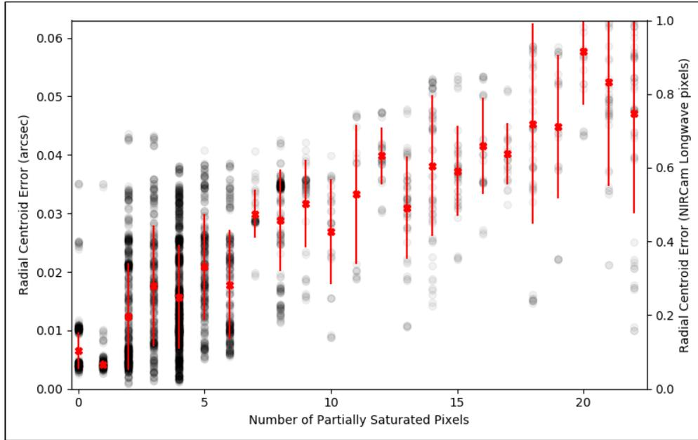
The number of pixels on the X axis is equivalent to the number of partially saturated pixels reported by the ETC. The red x's and error bars show the mean and standard deviation of the centroiding error. Note that fully saturated pixels begin to occur at limits described on the [ETC NIRCam Target Acquisition](#) article.
