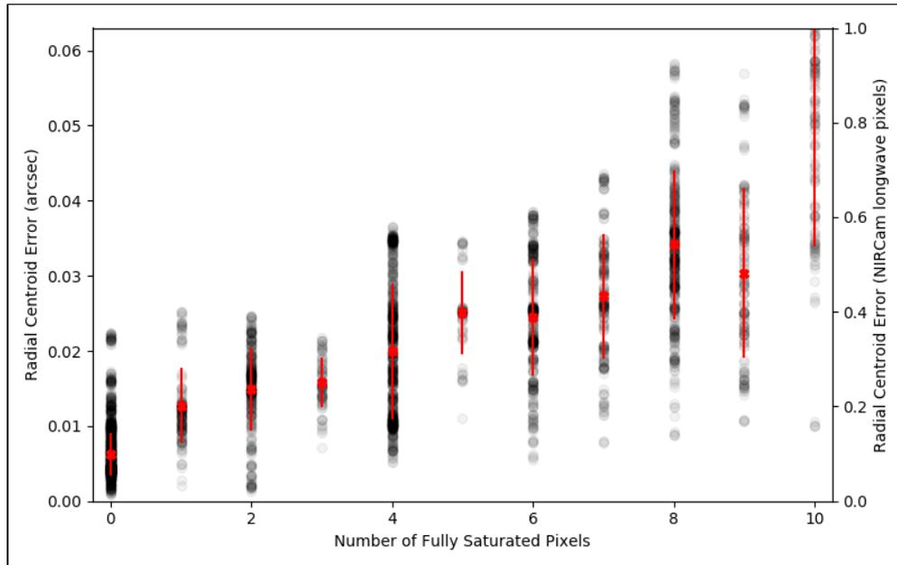
*The number of pixels on the X axis is equivalent to the number of fully saturated pixels reported by the ETC. The red x's and error bars show the mean and standard deviation of the centroiding error.*
