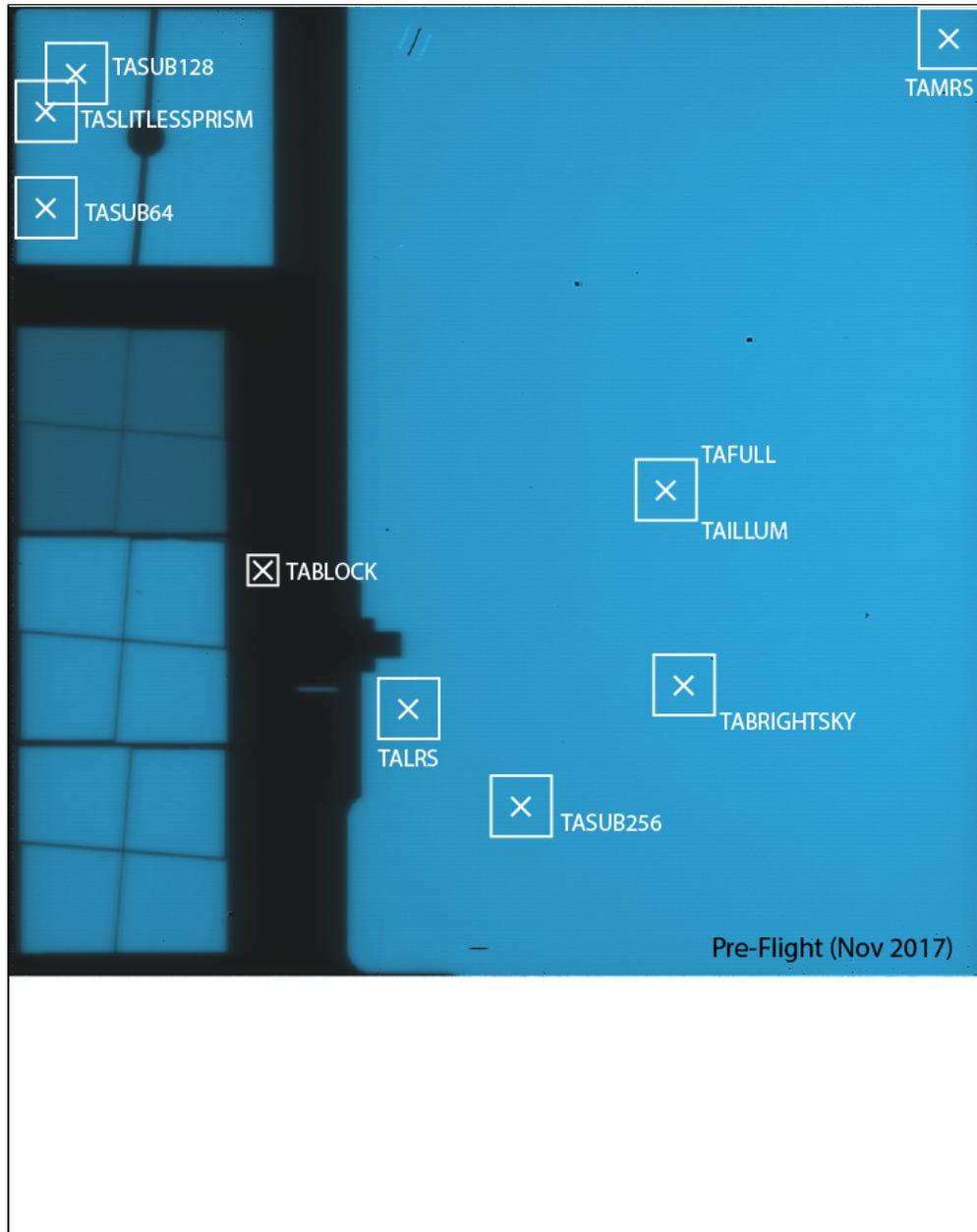
*The box labeled "TALRS" in the imager region is where the LRS slit target acquisition  $64 \times 64$  pixel region of interest (ROI) is located. The reference point is taken to be the midpoint of this ROI.*
